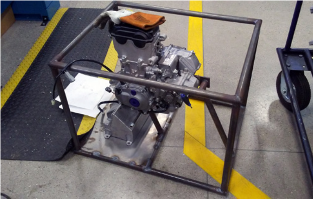
ABOVE: Our new Yamaha YZ450f engine, mounted in the portable test frame we built for it.
