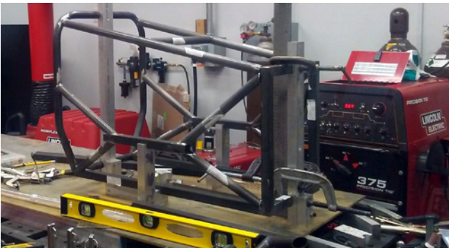
Frame under construction in the weld shop.
